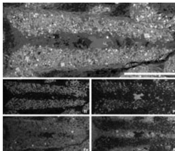
Figure 15. Backscattered electron micrograph of a near-complete *Volborthella* specimen from the southern Salt Spring Hills. Elemental maps below show distribution of four major elements, mapped using energy dispersive X-ray spectroscopy (EDS); light regions on the maps correspond to titanium (Ti, indicating ilmenite), phosphorus (P, indicating zircons), iron (Fe, indicating both ilmenite and iron oxides), and aluminum (Al, indicating clays). Scale bar = 1 mm.
